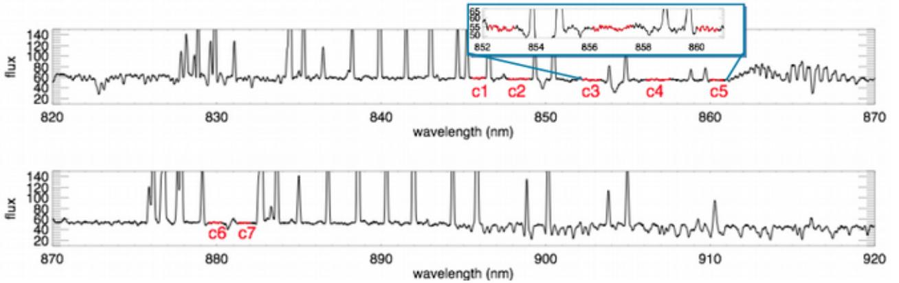
**Figure 2:** Sky spectrum from 820 to 920 nm obtained after combining 72 sky fibers. OH emission lines and atmospheric absorptions, i.e., telluric lines, can be seen almost everywhere. Only a few relatively clean continuum regions are left with the red c1 to c7 regions selected for further analysis.
